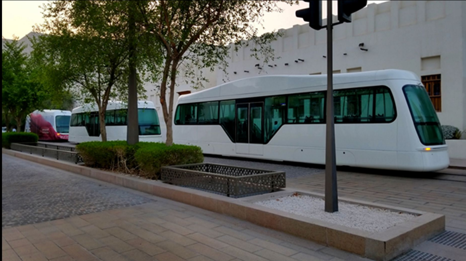
Three trams in autonomous coupling mode 1 x driver, 300 passengers
